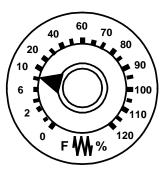
The rotary switch with 23 latched positions enables you to decrease or increase the *programmed* feedrate value "F "(corresponds to 100%).
