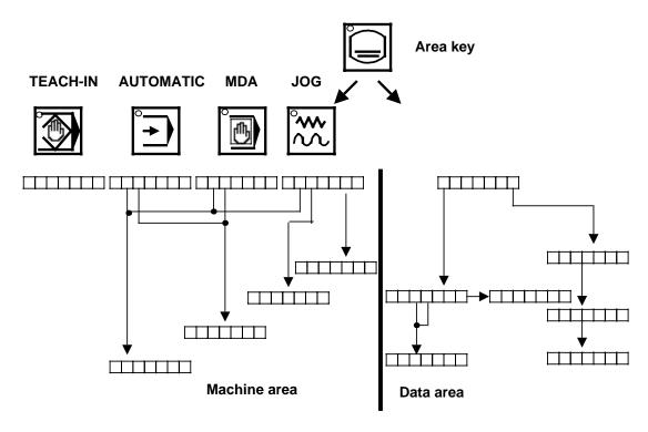
Using the area key, it is possible to branch to the data area's **basic menu** from any menu in the machine area.
